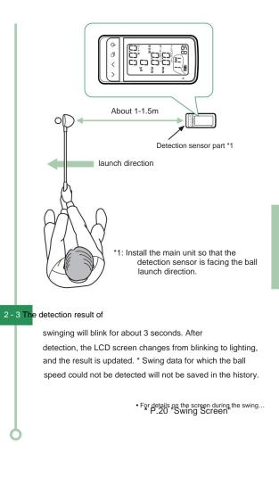
Images may not be displayed correctly in the following cases.•If the trajectory of the ball is high (the launch angle is large) or if it deviates to the left or right, it may not be possible to detect the ball speed. A club with a large loft angle has a large launch angle, so it may not be possible to detect the ball speed.
